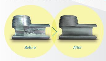
The thermal deburring is a system aimed at the elimination of burrs on the components made of oxidable materials and that come from specific processes (mechanical, die-casting, etc). The process uses, according to a chemical-physical principle, the heat generated from the ignition of a suitable combustible mixture, just as in the case of heat engines.
